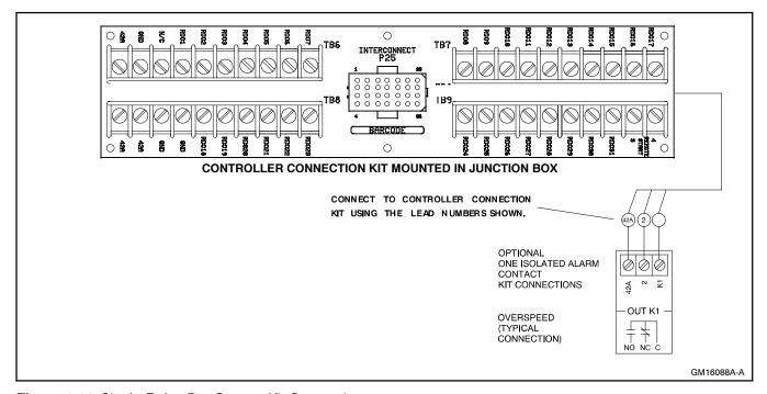
Figure 6-31 Single-Relay Dry Contact Kit Connections
